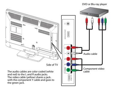
3 Connect an audio cable (not included) to the L/R (audio in) jacks on the side of your TV and to the L/R AUDIO OUT jacks on the component video device.
